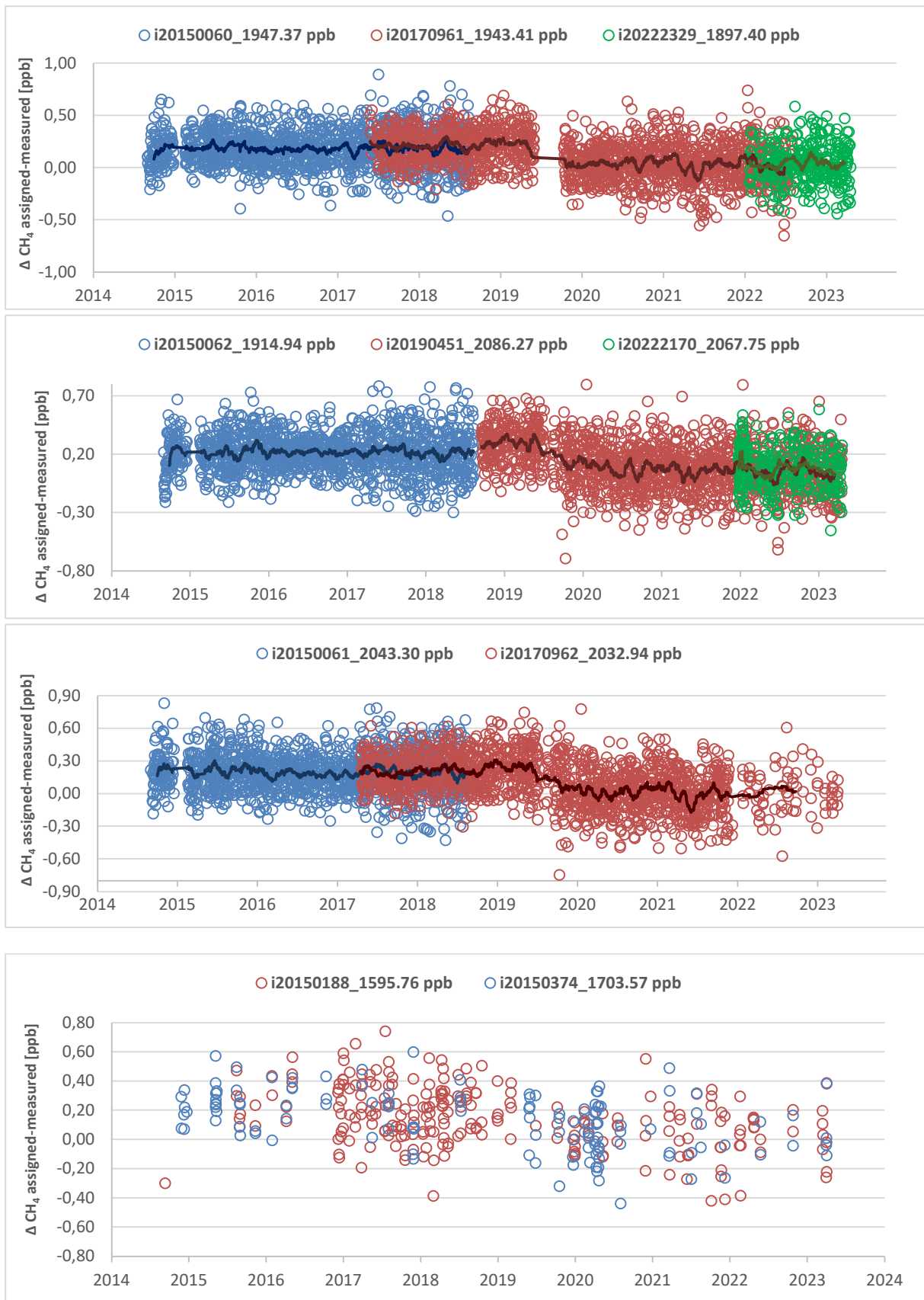
FIGURE 13: TIME SERIES OF THE CH 4 OFFSET OF TARGET MEASUREMENTS TO THEIR RESPECTIVE ASSIGNED VALUES. The dark line represents a 30 points-running mean.
