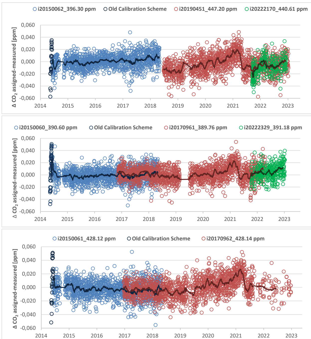
FIGURE 4: TIME SERIES OF THE OFFSET OF CO 2 TARGET MEASUREMENTS TO THEIR RESPECTIVE ASSIGNED VALUES. The dark lines represent a 30 points-running mean. (Three outliers in January 2018 and January 2019 have been flagged out for i20150060, i20150061 and i20150062 for a more explicit visualization).
