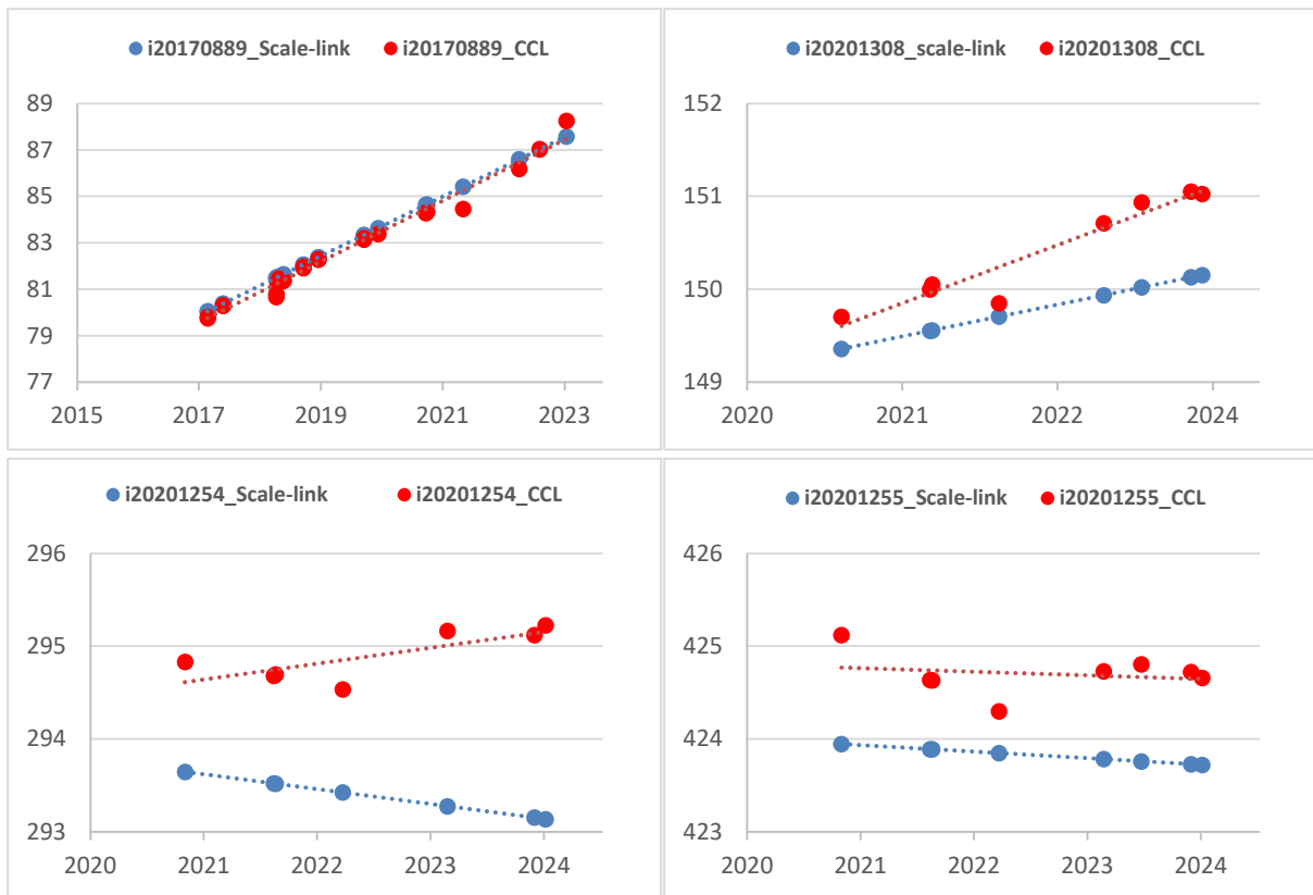
FIGURE 23: SECOND SET OF SECONDARY CO STANDARD: ASSIGNMENT RECORD AGAINST FCL'S PRIMARIES (RED DOTS) AND FCL'S OLD SET OF SECONDARIES (BLUE DOTS) (VALUES IN [PPB]).
